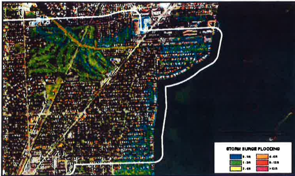
Figure 5 This map indicates the maximum flooding that could be expected from storm surge associated with a category 1 hurricane making landfall near Miami Shores during high tide under 2018 sea level conditions.
